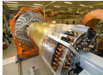
Figure 4: Insertion of barrel SCT into barrel TRT; the OTE is visible surrounding the barrel SCT, as well as the services on the ISSS (foreground).
