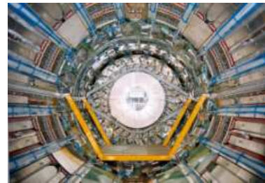
Figure 8: The barrel ID installed in its final position inside the electromagnetic calorimeter cryostat bore.
