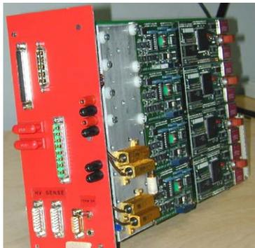
Figure 1: The Test Fixture developed by Torino-INFN and CAEN for the quality control on A4601H production
