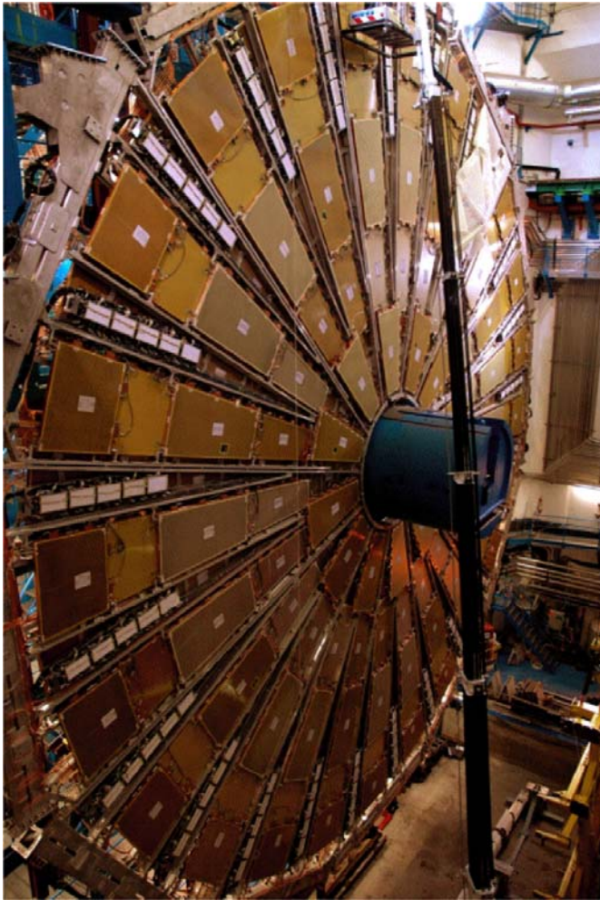
Figure 8: The completed M1 station of TGC in the ATLAS pit (Sept., 2006)
