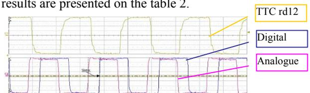
Figure 12: recovered clocks from the three transmission schemes
