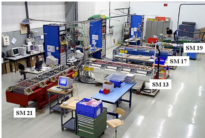
Figure 2: The electronics integration area at CERN. Installation can proceed in parallel on up to four supermodules.
