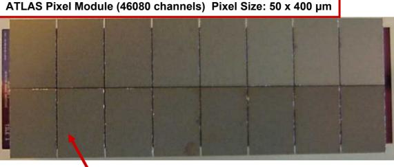
Flexible PCB Front-End ICs Sensor (between PCB and IC) (x16) Module Controller Chip (MCC)
