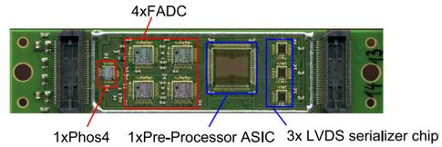
Figure 2: The Multi-Chip Module
