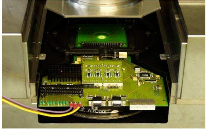
Figure 5: The PPrASIC test-hardware mounted in the wafer-probe station.
