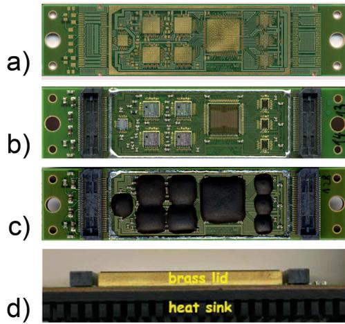
Figure 7: MCM assembly steps: a) MCM substrate; b) MCM with all dice bonded on substrate; c) MCM with glob-topped dice; d) MCM with brass and heat sink (side view).
