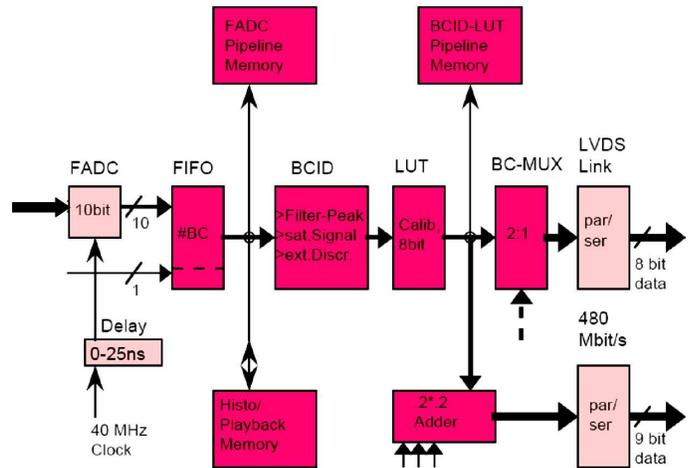
Figure 3: Block diagram for the processing of one calorimeter channel on the MCM
