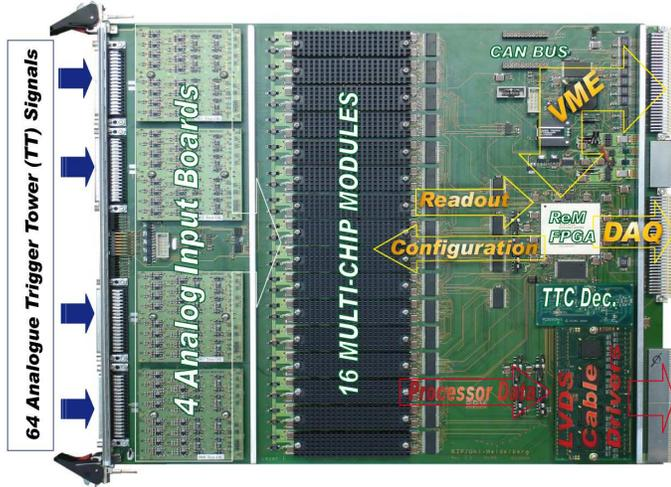
Figure 1: The Pre-Processor Module
