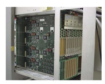
In order to check possible transmission errors, a checksum is generated in the Input Cards on each fragment, transferred to the Builder Card, and compared with a checksum being generated.
