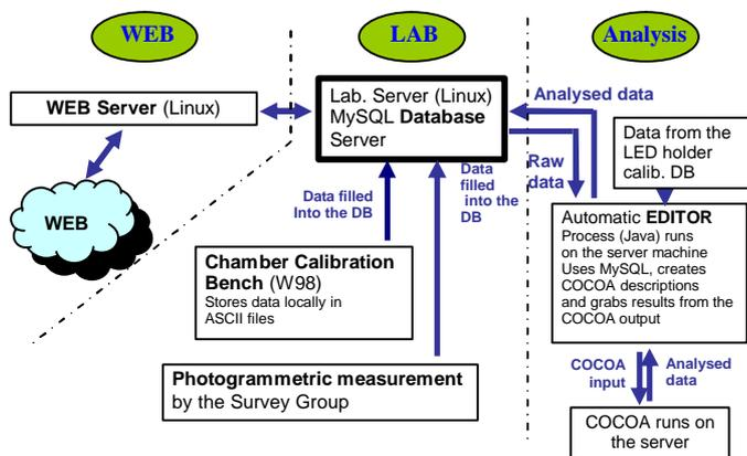
Figure 4. Data flow during the muon chamber calibration
