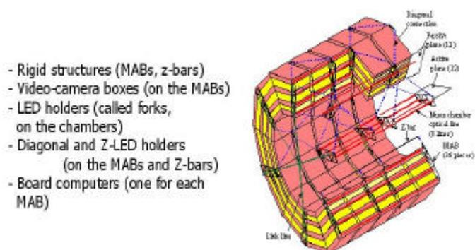
Figure 1. CMS Barrel Muon Alignment scheme
