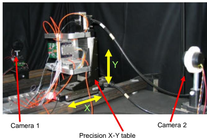
Figure 2. Calibration bench for the LED holders.
