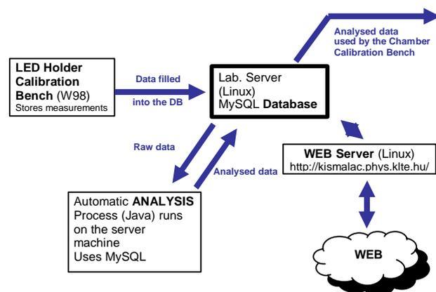
Figure 3. Data flow during the LED holder calibration [5]
