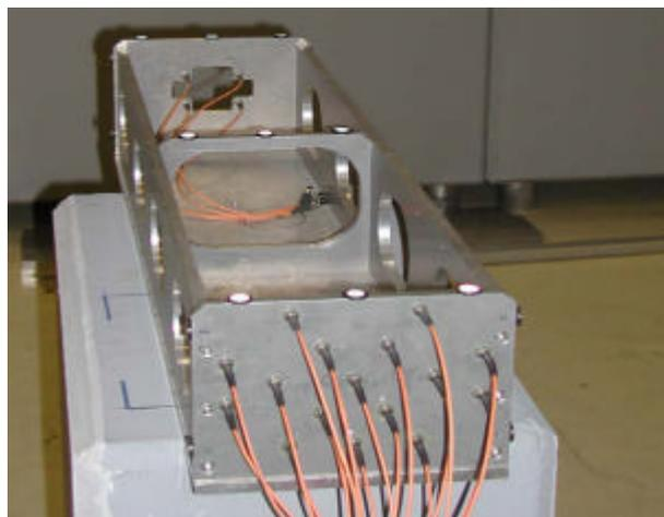
Figure 6. Camera calibration bench
