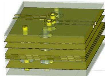
Figure 9: Differential vias geometry in MWS
