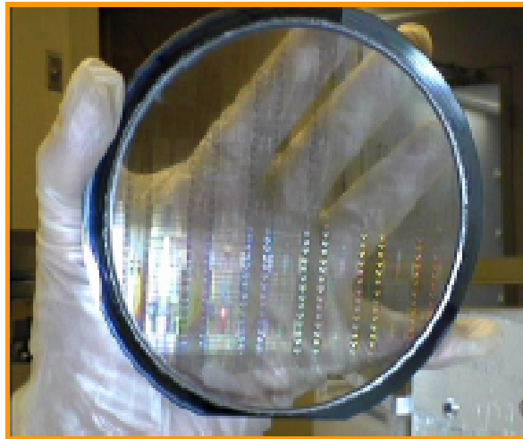
Thinned wafer mounted on Quartz handle wafer (MIT Lincoln Labs)
