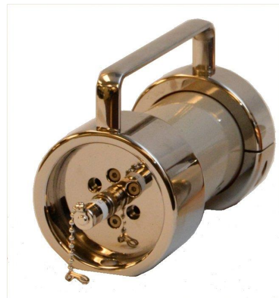
BC-60 Faraday (provides independent absolute measure of the beam charge)
