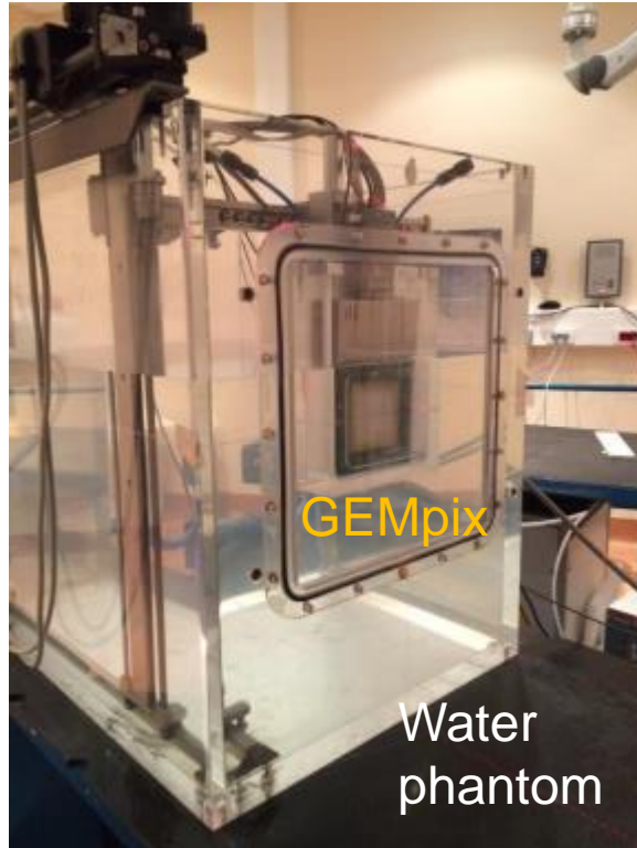
GEMPix inserted in a water phantom
