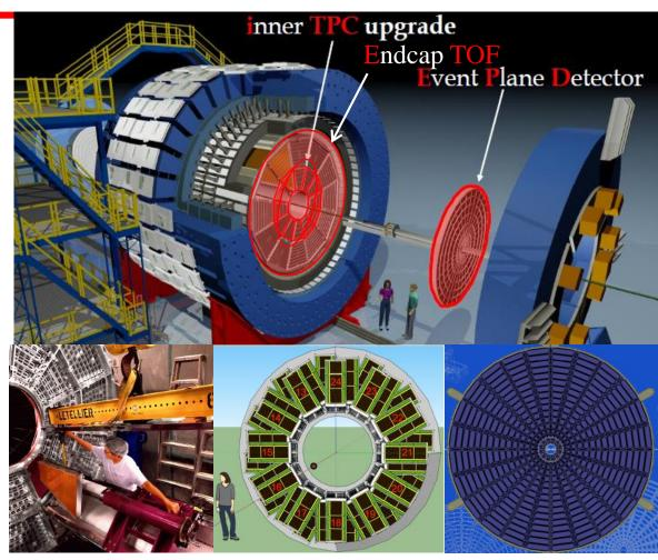
Upgrade to TPC, new end-cap TOF, new forward trigger
