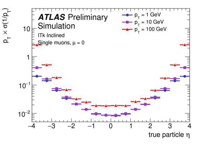
• The benefit of high precision measurements of the all-silicon tracker of the ITk should yield a better momentum resolution than the current ATLAS ID
