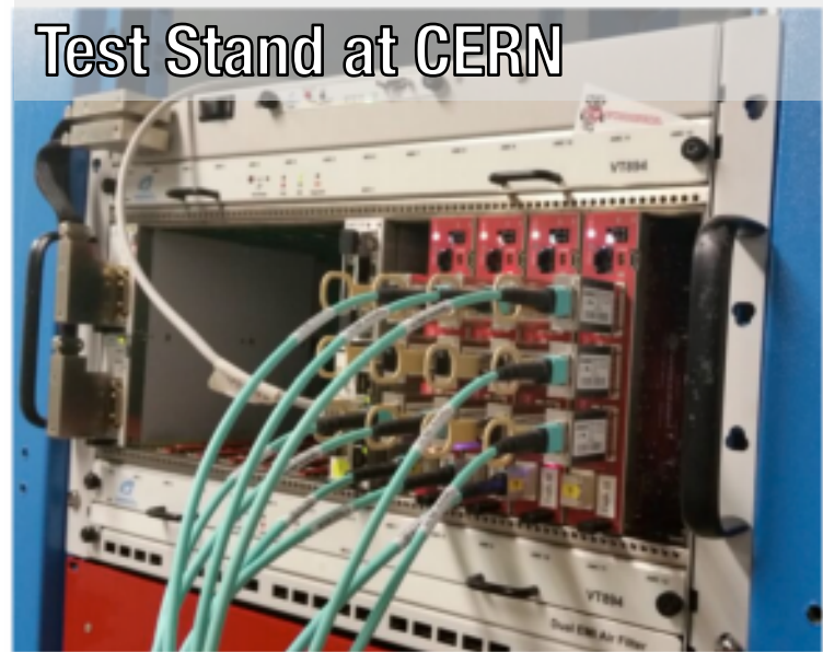
CTP7 Boards from Univ. of Wisconsin Currently used in CMS L1 trigger
