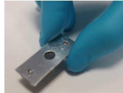
Self-supported thin film mounted on the holder for measurements
