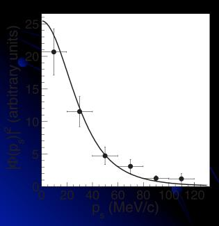
Solid circles: measured momentum distribution of the neutron inside deuteron using the  ${}^{2}H({}^{18}F,a{}^{15}O)$ n reaction
