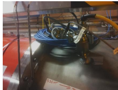
Testing EHBS at P8 (UA87; QYC01&QYC04) crates with long cables (50m&100m) and external load.
