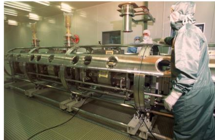
Figure 2.1: LHC cavity module being assembled in a clean-room [1]
