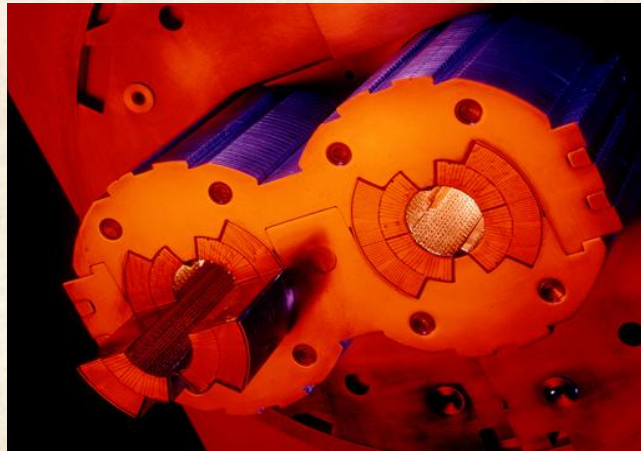
NbTi LHC standard dipoles, 8.3 T
