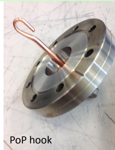
23 cm-long antenna for beam pipe
