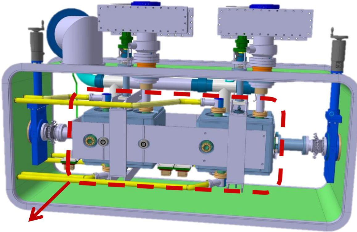
Magnetic & thermal shielding
