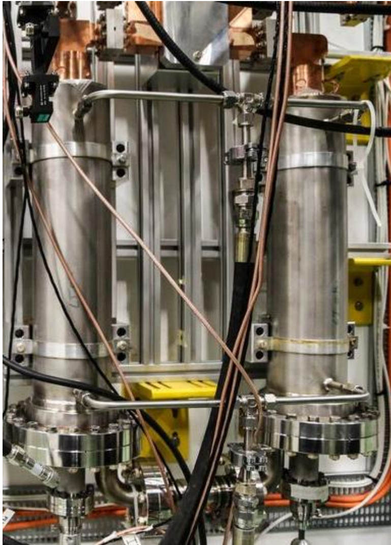
Pulse Compressor (same as Xbox-2 but with lower coupling) See: Matteo Volpi this pm.
