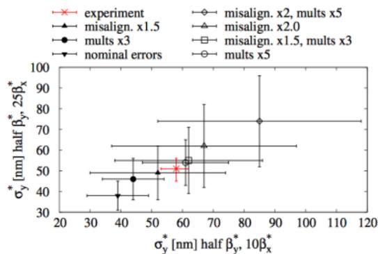
FIG. 11. The IP beam sizes measured in ATF2 (red) and obtained with simulations without the orbit correction (black) for half  $\beta_y^*$ ,  $10\beta_x^*$  and half  $\beta_y^*$ ,  $25\beta_x^*$  optics.
