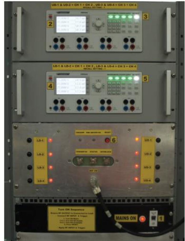
Figure 2.6.1 The turn on sequence is mentioned on the front panel of the amplifier. The Turn ON and Turn OFF sequence are detailed on next page.
