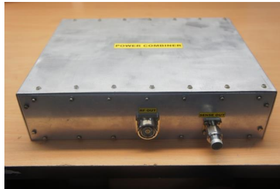
High Power Microwave combiner (microstrip line based) 8:1
