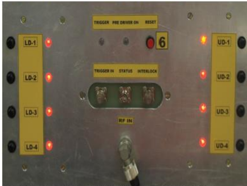
Figure 2.4.1 The amplifier controls, interlocks and indicators are present on the front panel
