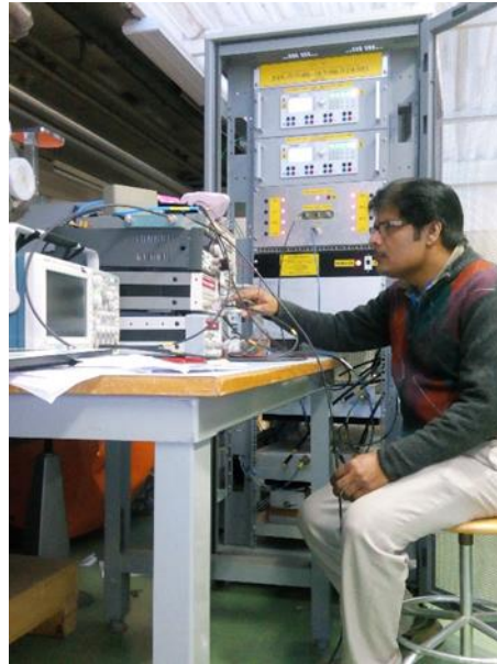
Test set up at CERN for testing the RRCAT 20kW SSPA
