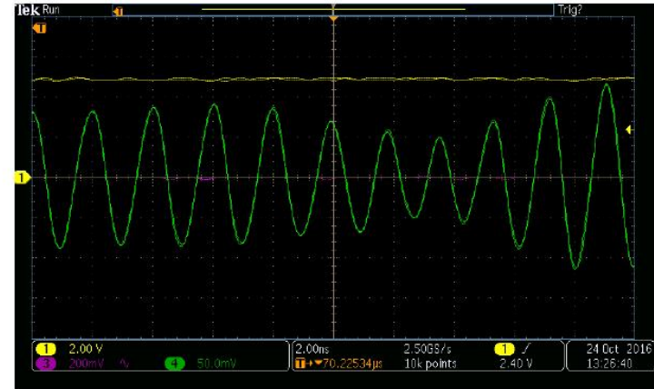
Figure 11: Phase shift of the SSAP output signal, 70.8 dB attenuated at 499.75 MHz and 7 dBm input power at the amplifier. Gradual phase shift process gets visible, transmission time 8 ns. The phase shift causes amplitude variations of around -40%/-4 dB.
