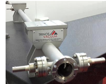
Damping ring kickers Prototype CLIC DR extraction kicker (Courtesy of C. Belver-Aguilar)
