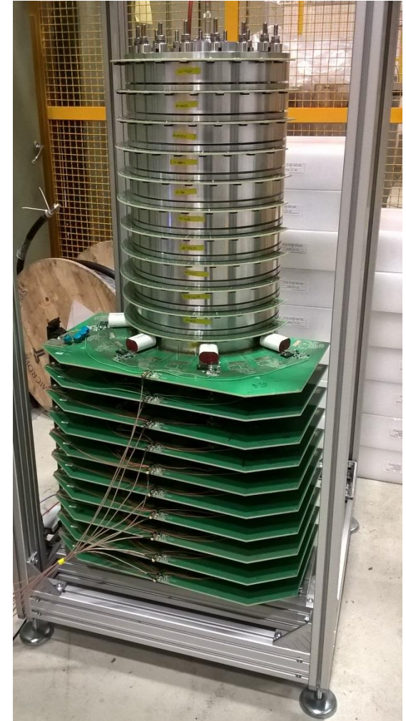
The first 20-layer inductive adder prototype at CERN
