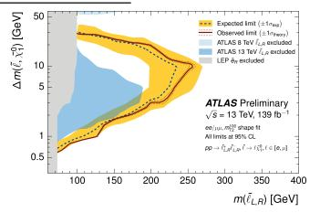
Exclude sleptons below 256 GeV at a mass splitting of 10 GeV, and extending down to a mass splitting of 590 MeV at the LEP limit
