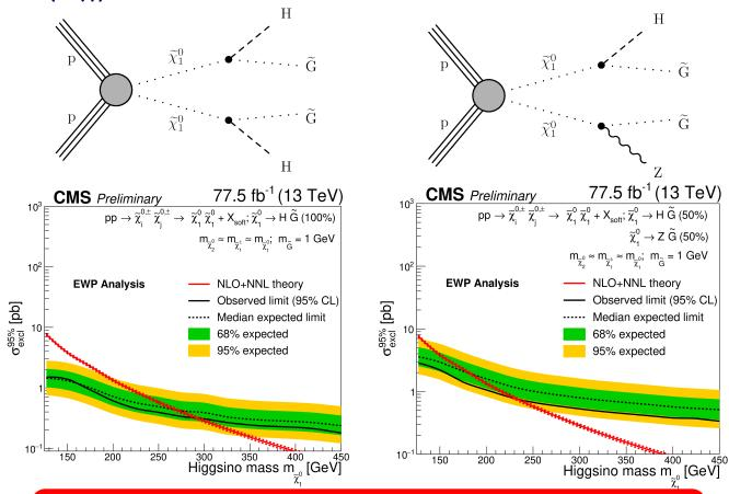
Exclude neutralinos below 300 GeV (100% decay to H) and 180 GeV (50% decay to H and 50% decay to Z)
