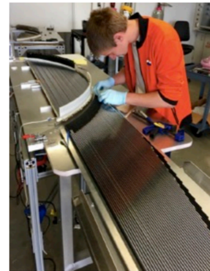
Panel: Straw Installation
