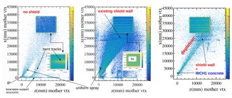
Concrete wall around RICH1 "qualitatively" explains the depletion of hits in upstream region, seen in the BG measurements
