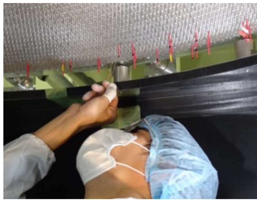
Wire stringing and tension measurement for 19,548 wires were carried out in a half year.
