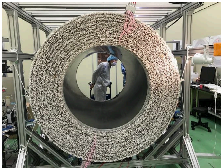
Cabling from feedthroughs to HV, RO & GND
