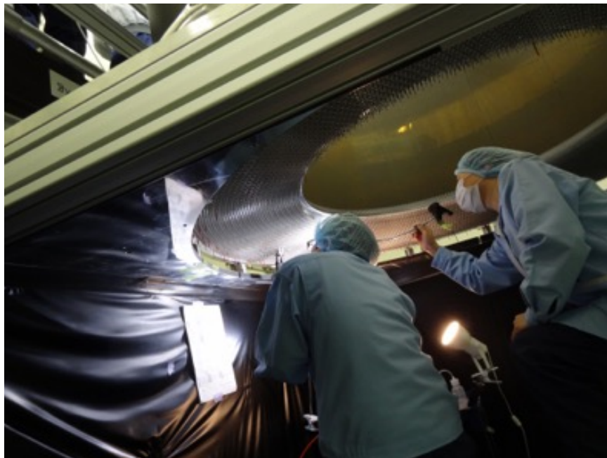
Wire stringing and tension measurement for 19,548 wires were carried out in a half year.
