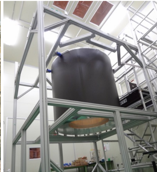
Outer structure was transported to a KEK assembly hall, and set on a wire stringing cradle.
