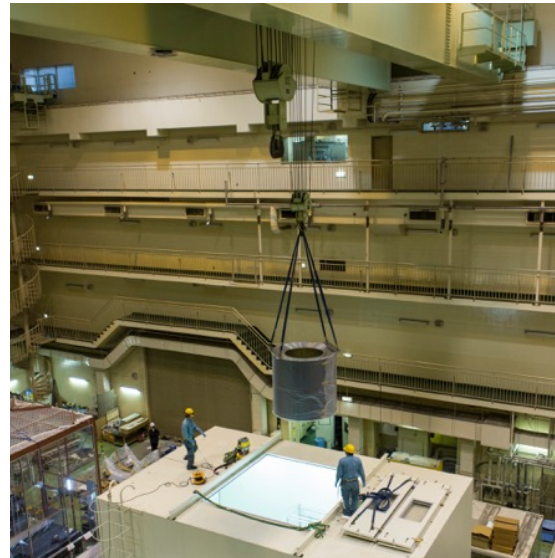
Outer structure was transported to a KEK assembly hall, and set on a wire stringing cradle.
