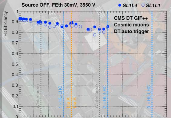
The hit efficiency was weekly measured with no background (source off) during the irradiation of the chamber. For a HV of 3550V, the hit efficiency is reduced <10% after integrating 2xHL-LHC expected luminosity.
