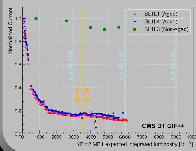
The currents in the aged layers (SL1L1, SL1L4) were monitored during the irradiation period. The currents on the non-aged layer SL1L3 are used as reference. Most of the drop of currents is observed during the first 1000 fb<sup>-1</sup> of accumulated luminosity.
