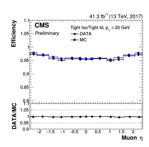
Efficiency of muon identification (ID) and isolation criteria measured with a Tag-and-Probe **method** [4] using events with dimuons from  $J/\psi$  or Z decays collected with triggers requiring the presence of, at least, a single muon.
