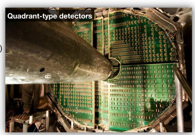
Only the CPC readout electronics will be upgraded during LS2
