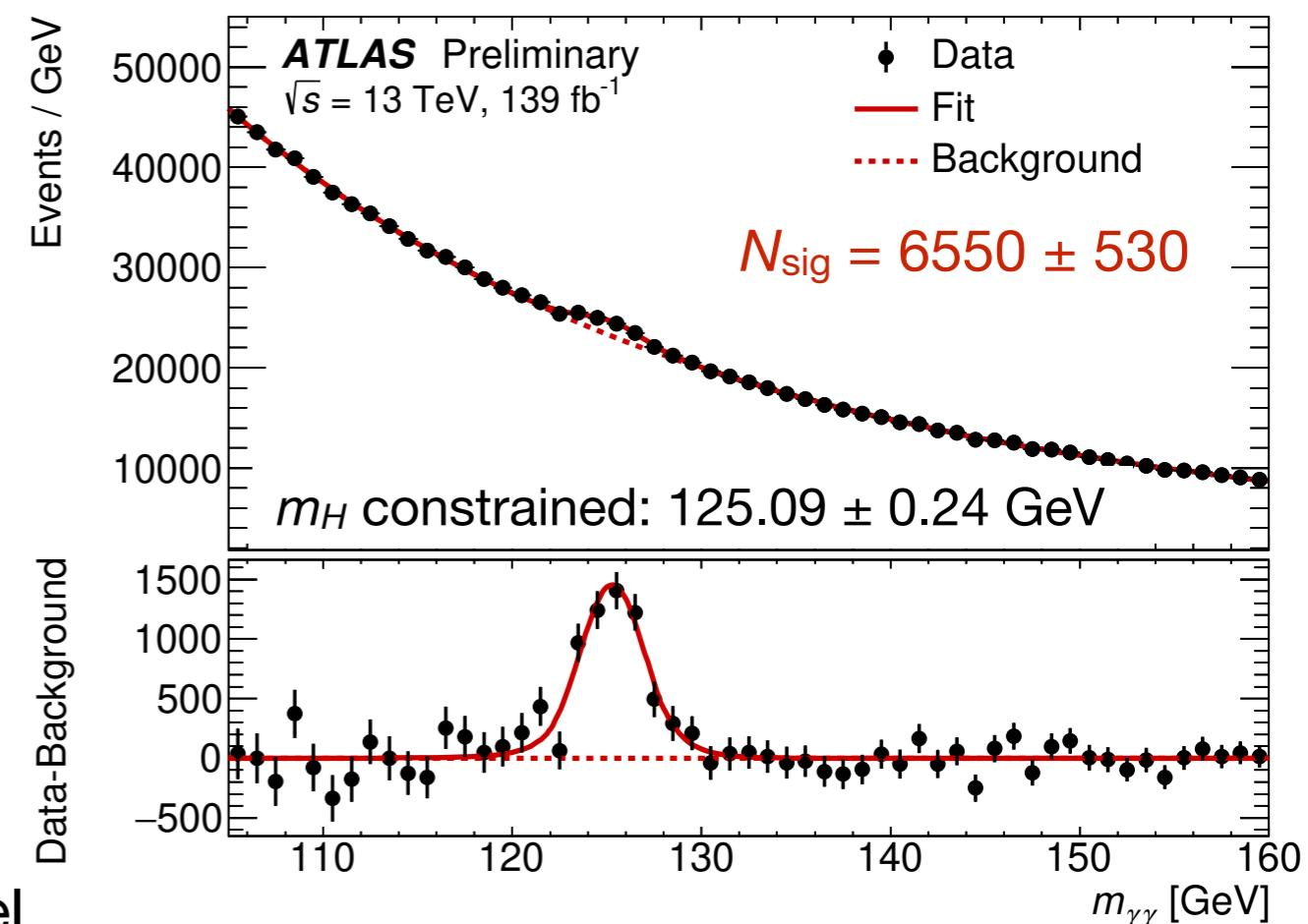
$$\sigma_{\text{fid}} = \frac{N^{\text{sig}}}{c_{\text{fid}} \mathcal{L}_{\text{int}}}$$
