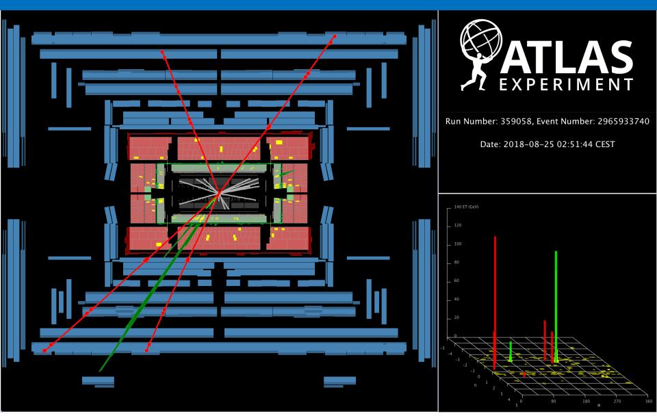
Invariant mass of the extra di-muon in the upper hemisphere is 91.5 GeV.
