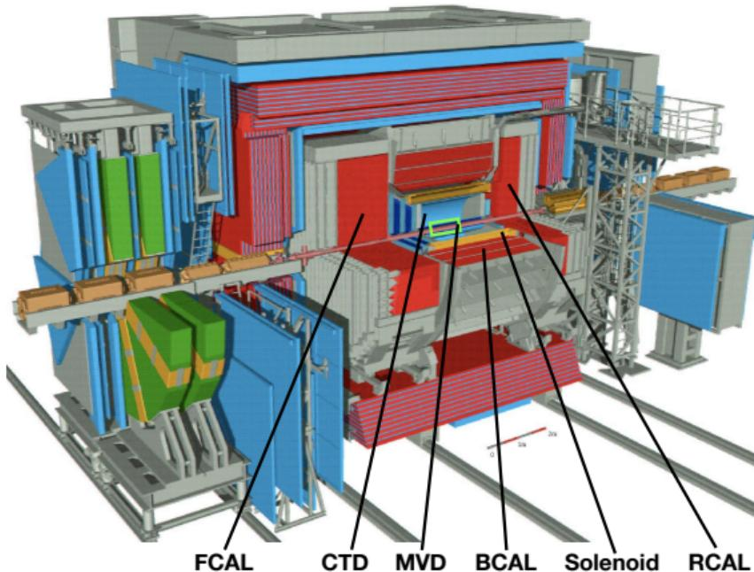
Charged particles are tracked in the central tracking detector (CTD) and micro vertex detector (MVD) in a 1.43 T magnetic field.
