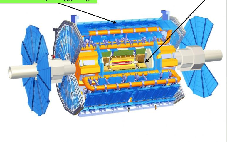
Muon Chambers with Improved Readout Granularity / Triggering.
