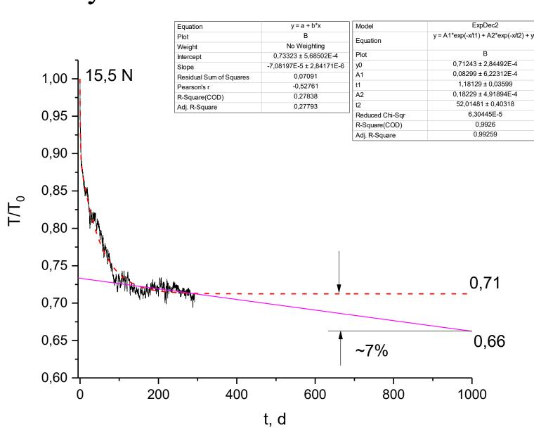
more realistic estimate, a linear approximation of the data's tail (starting from the 90th day) was made. The main result is that after 3 years (COMET straw tracker lifetime) the straw tension will be about 66% of initial. Taking this into account the optimal initial straw tension can be determined. In the COMET case, it is 1.23 kgf.
