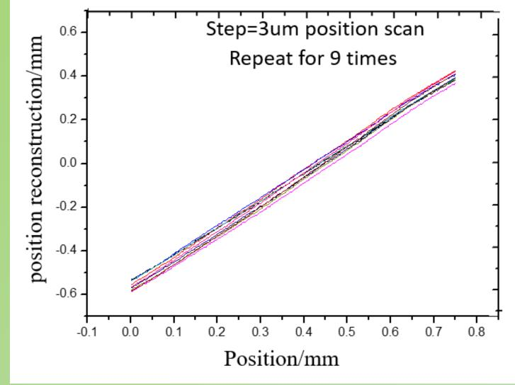
Fig.2 a linear relationship between the real position and the reconstructed position
