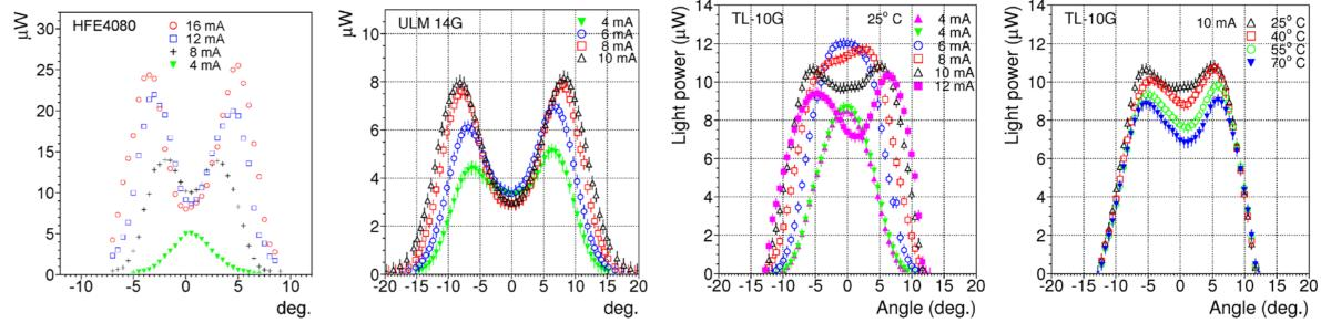
Far-field patterns of VCSELs at various DC currents. The Truelight 10 Gbps type was tested in a Chamber for temperature dependence with the light power scanned though a open window (picture).
