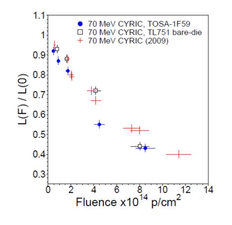
Light attenuation of irradiated VCSELs is approximately linear to proton fluences tested to 1x10<sup>15</sup> (70 MeV) p/cm<sup>2</sup> [1].
