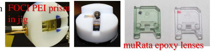
Durability of the FOCI prism assembly was tested at 85°C/85% RH. The assembly in die/wire bonds and UV-glue on PCB endured burn-in of 4000 hours, in a stable light coupling condition.
