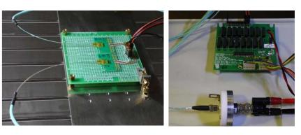
Light power of the FOCI packaged VCSEL is measured with the fiber connection to a PD in a jig.
