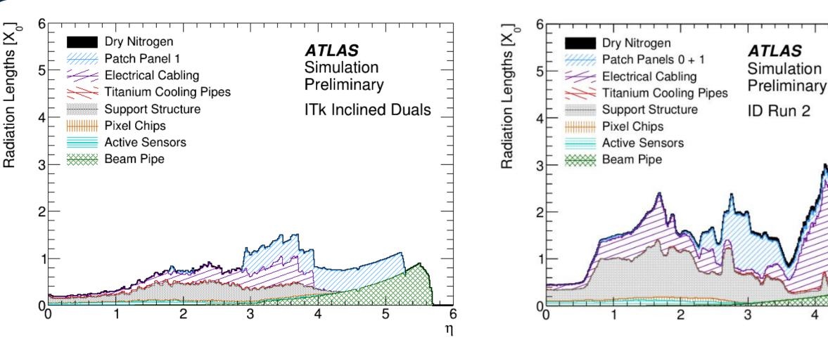
Material (in radiation lengths) vs η for the proposed ITk Inclined Duals layout [left] and the present Run 2 Inner Detector [right]
