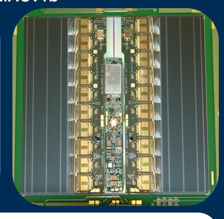
Modules have now been built using a prototype AMAC chip. All control, monitoring and autonomous interlocking functionality has been successfully demonstrated.
