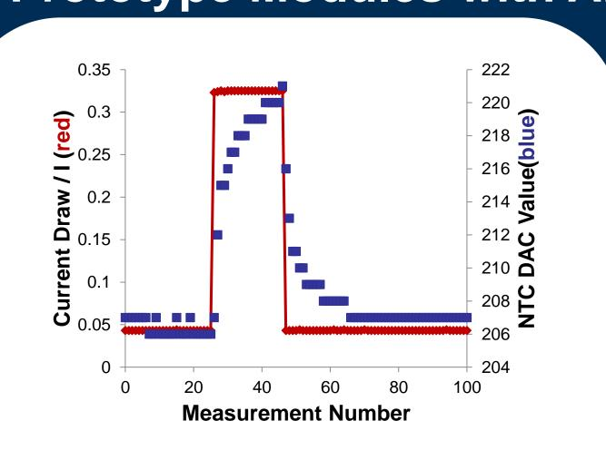
The current drawn by a module falls when AMAC disables the DC-DC converter in response to the temperature having exceeded the set threshold.
