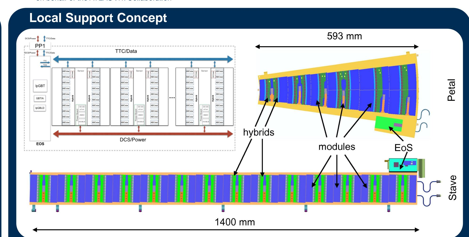
Strip tracker built up from staves (barrel) and petals (end-cap); carbon fibre local supports with integrated cooling pipes, covered with polyimide flex circuits providing cooling, powering, control and readout.
