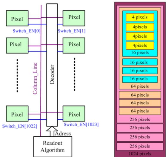
Fig.4 Readout architecture of one column Fig.7 Hierarchical decoder
