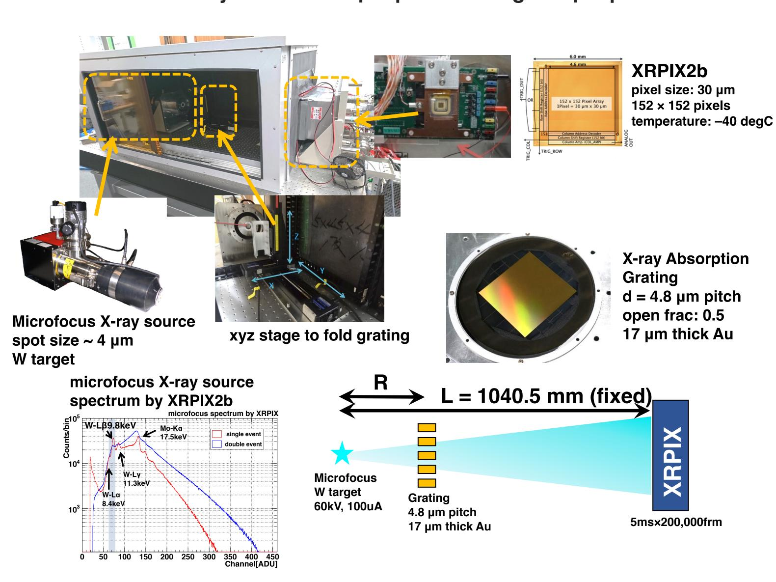
The period of X-ray Talbot interference fringes @R = 235 mm is expected to be 0.7 pixel (21 μm). To obtain sub-pixel resolution, we employ the charge sharing analysis.
