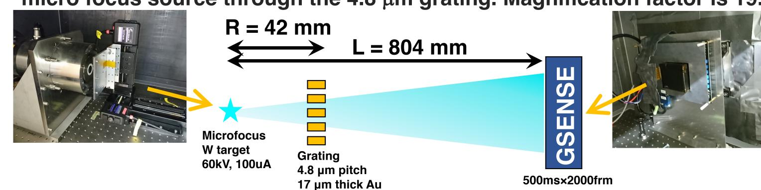
In this condition we could see 21 pixel period self image on GSENSE5130 without applying the charge sharing analysis.
