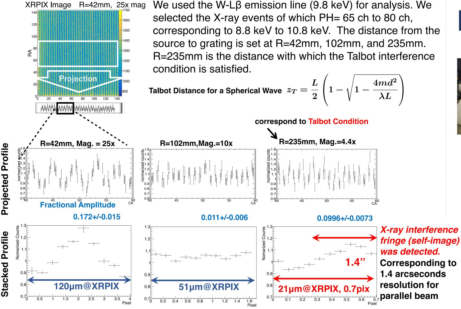
In this experiment, magnification of factor 4.4 helps us to detect the X-ray interference fringe. X-rays from celestial objects is parallel, and no magnification is expected. We thus need finer pixel detector of whch pixel size is similar or smaller than the grating pitch.
