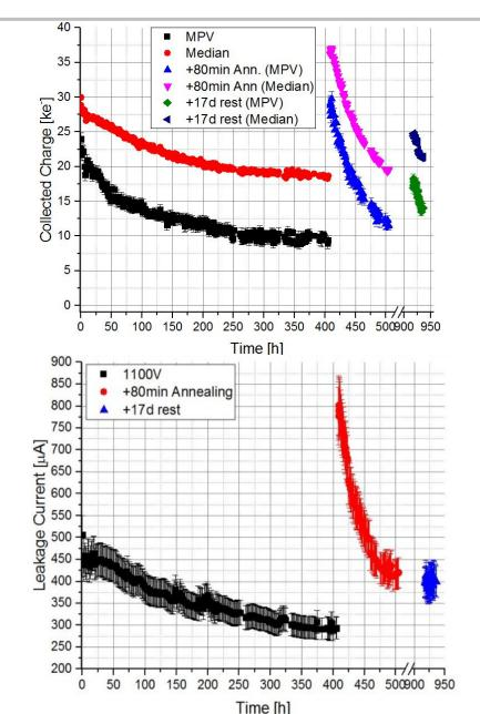
2x10<sup>15</sup> n<sub>eq</sub> cm<sup>-2</sup>, 5000 min annealing at 60°C, sensor in charge multiplication
