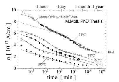
• Damage rate α proportional to leakage current
