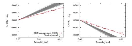
• Measured Q-spread from IR- $b_4$  at 40cm  $\sim \frac{1}{3}$  of that generated by MO (2016)
