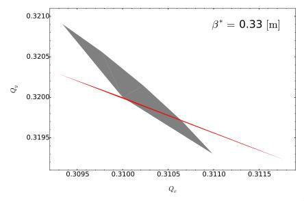
Stability diagram at  $\beta^* = 33 \text{ cm}$  with & without IR b<sub>4</sub> errors Simulations and plot by Xavier Buffat (CERN)
