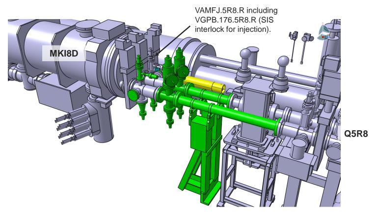
**EYETS** - Two new NEG cartridges of 400 l/s each (nominal speed for H<sub>2</sub>) will be integrated in new modules of vacuum sector I5R8.
