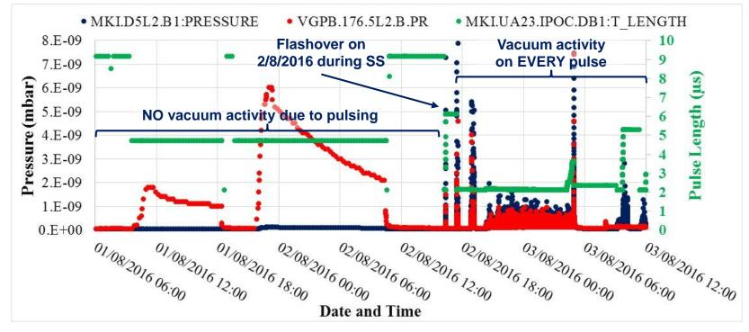
August 2016 to TS3 2016: MKI2D operated with ~3 µs field pulse flattop.
