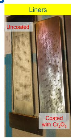
Planned to put a liner in the SPS during EYETS, with a  $Cr_2O_3$  coating: two sets of liners now coated;
