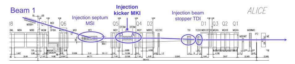
During LS1, the vacuum systems on the interconnects between MKI magnets were upgraded: ✓ Interconnects NEG coated;
