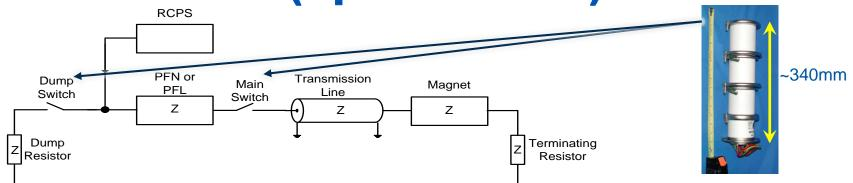
One Main Switch (MS) thyratron erratic during resonant charging for injection on 2/9/2016: 876 circulating bunches of which ~210 miskicked.
