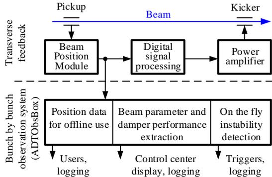
Figure 2: Integration of the ADTObsBox into the transverse feedback system.
