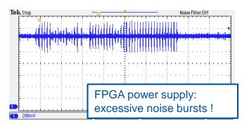
**Investigations:** Found power supply *shortcut* through FPGA. High level of *noise* on the FPGA power supply was also noticed. => Will be corrected during EYETS.
