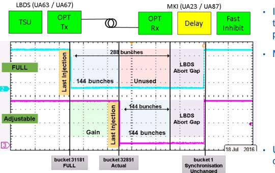
Implemented during TS1 in 2016, to allow the last injection of 144b, due to TIDV problem and intensity limitation in SPS.
